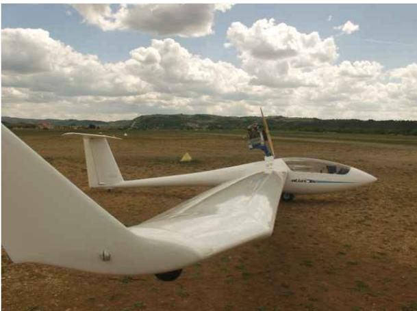
**TST-10M Atlas** is a single-seat self-launcher with a retractable power unit, suitable for thermal flights and wave or ridge flights. The aircraft offers easy handling and the capability of independent take off.
