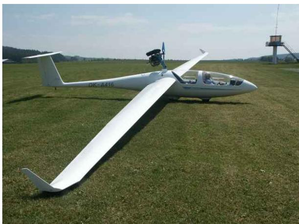
**TST-14M Bonus** is a two-seat motorized composite light self-launcher with a retractable power unit, suitable for thermal flying, wave or ridge flights and for clubs and flight schools. The aircraft also offers easy handling and the capability of independent take off.
